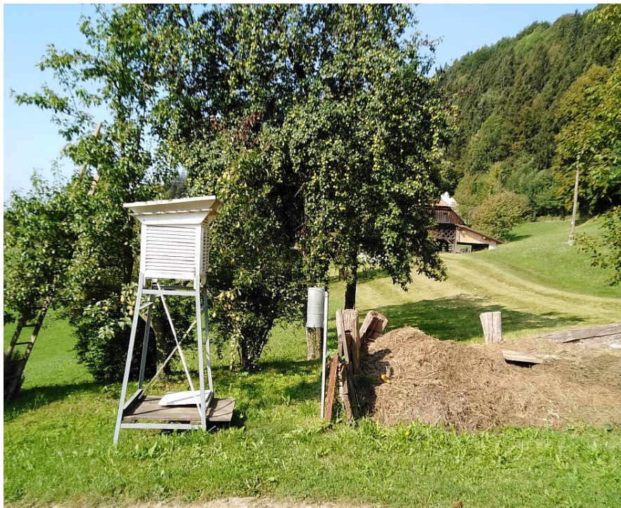
Slika 2. Padavinska postaja in elektronski zapisovalnik temperature in vlažnosti zraka (v meteorološki hišici) v Čemšeniku, slikano septembra 2020 (vir: arhiv ARSO) Figure 2. Precipitation station and data logger for measurement of air temperature and humidity (in radiation shield) in Čemšenik, photo taken in September 2020 (from: archive ARSO)
